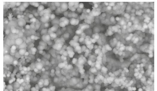
Under 2500x magnification the detailed morphology of hydroxyapatite crystals becomes more evident through scanning electron microscopy.<sup>5</sup>
