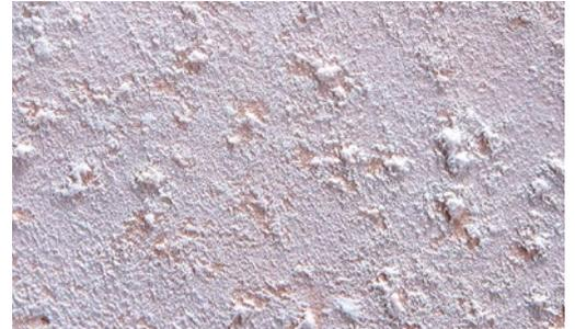
At 3.5x magnification the material's surface shows the distinct development of hydroxyapatite crystals.<sup>5</sup>
