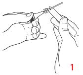
Place one or more silicone stops on the tip of the corresponding needle using the key.
