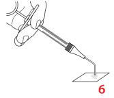
Prepare the repair material on a glass tab and transfer the required quantity of material into the filling well. Thrust the tip (of the needle) into the repair material several times so that it is filled.
