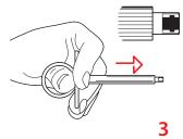
Press the piston of the MAP Syringe so that the bayonet tip appears.
