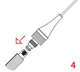
Fit the plunger bayonet counter system and release the syringe piston.
